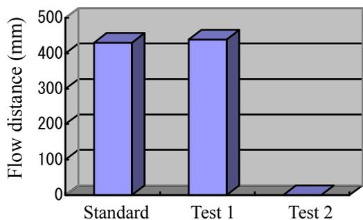
Fig. 7 Change of flow distance with the addition of fly ash
