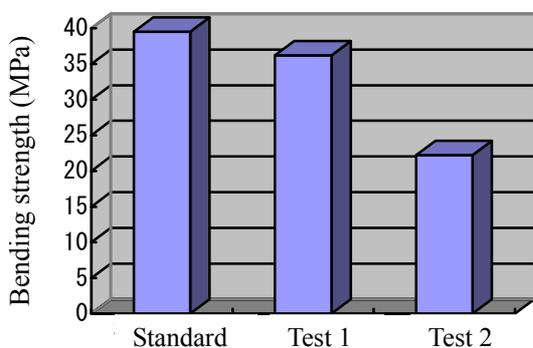
Fig. 8 Change of bending strength with the addition of fly ash
