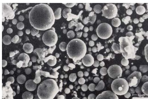
Fig.4 Electron micrograph of fly ash
