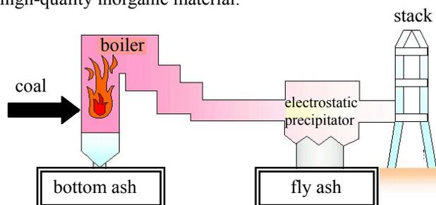
Fig.2 The place where coal ash was captured
