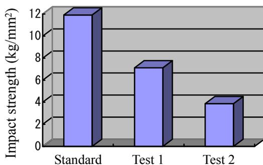
Fig. 9 Change of impact strength with the addition of fly ash
