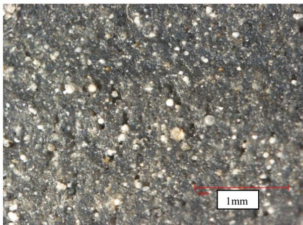
Fig. 5 Sectional picture of rubber filled fly ash
