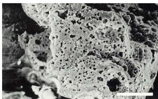
Fig.3 Electron micrograph of bottom ash
