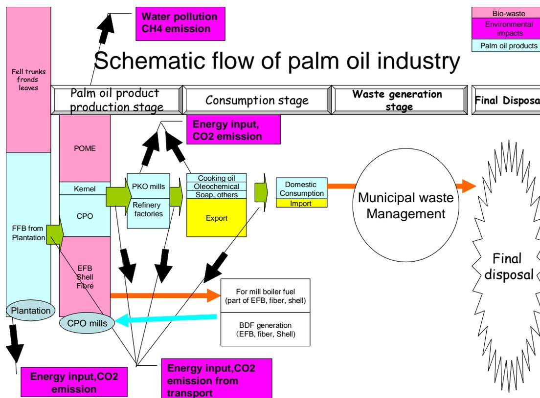
Fig.1. Schematic flow of palm oil industry
