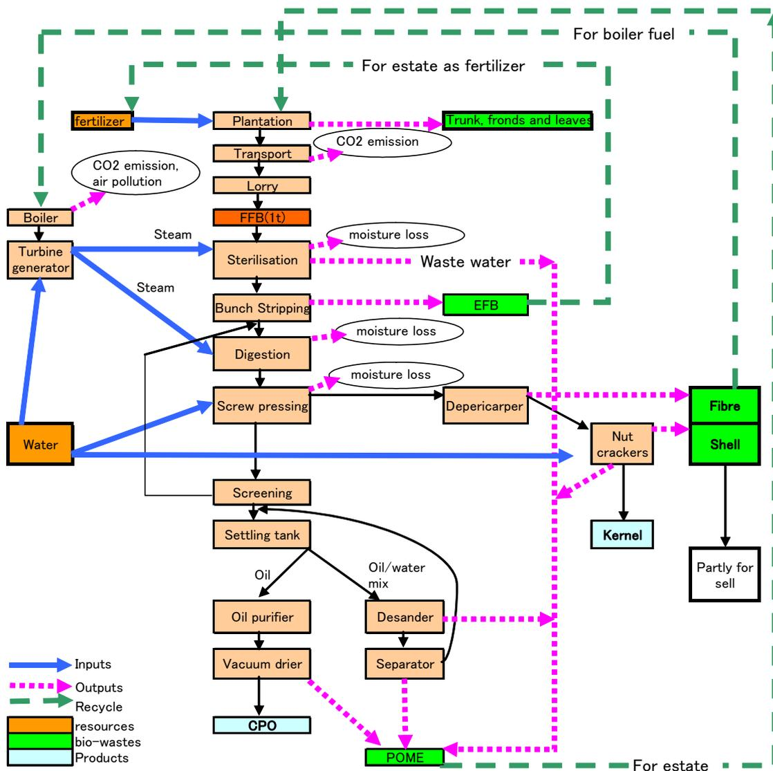
Fig.3. Production process of a CPO mil in Indonesia
