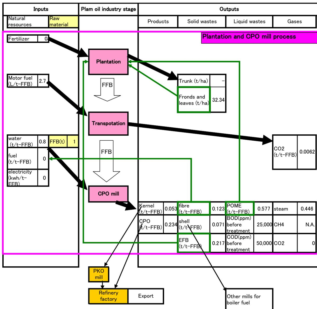
Fig.4. Material balance of typical palm oil plantation and CPO mil in Indonesia (per one t-FFB basis)
